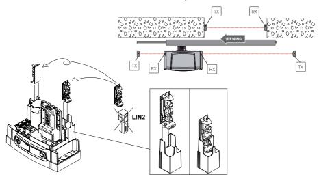
Additional photocells can be installed inside the gearmotor casing of Ditec NEOS, to protect both opening and closing movements by using the LIN2 photocell.
